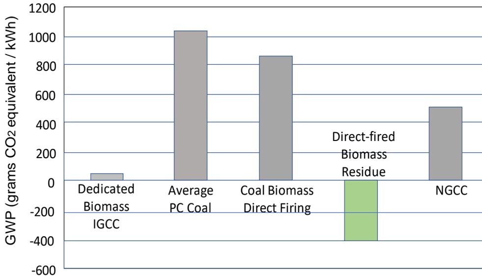
**Figure 2.** Life cycle assessment <sup>[3]</sup> shows that thermal conversion of biomass residue to energy results in a net reduction of greenhouse gas equivalent emissions because of the resulting diversion from landfill, where anaerobic decomposition would otherwise produce methane
